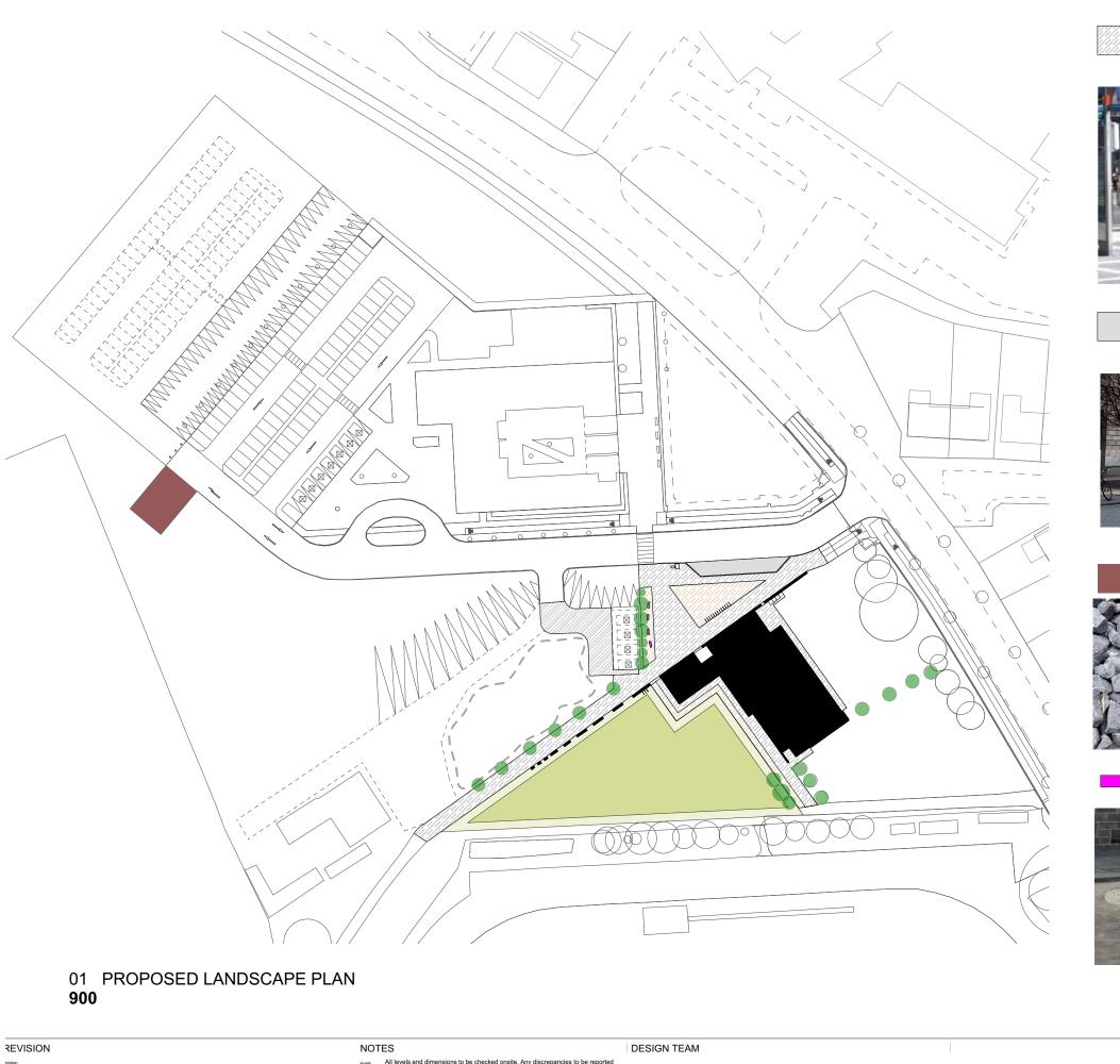
Plaza & Footpath 1700x450 mm limestone paving slabs content to architect's approval
